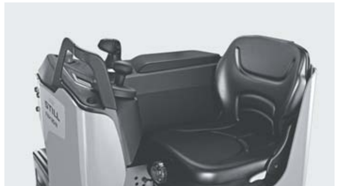
Cushioned driver's seat which can be adjusted to the driver's weight for maximum comfort
